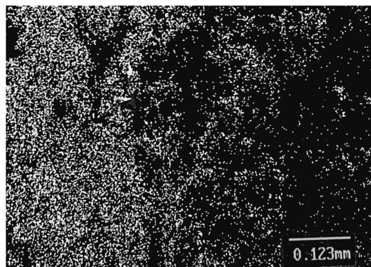
Fig. 5. Characteristic X-ray images of Si in the cross section of a typical sample.
